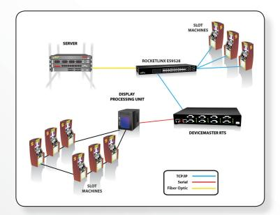
switch or facility network. Comtrol's DeviceMaster serial hubs may also be used in this layout, to bring legacy, serial-supported games into the primarily Ethernet-supported network. Whether a gaming facility updates a whole network simultaneously or implements gradual changes from serial to Ethernet communication, Comtrol's products support many different configurations for facility-specific solutions.
